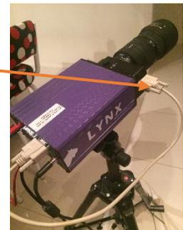
Screw antenna into **Linkgate remote** (Decradio). Attach to back of camera in C-box serial port and plug in red cable to red +Output. Hang remote as high as possible.
