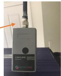
1.5. **Linkgate Activator** – attach (Encradio 500) antenna. Make sure this is charged up. Will hold its charge for many hours. Check charge by turning on and wait for beep, then press ON/OFF button quickly to get remaining percentage of usage time. Hold down ON/OFF button to turn unit on and off.
